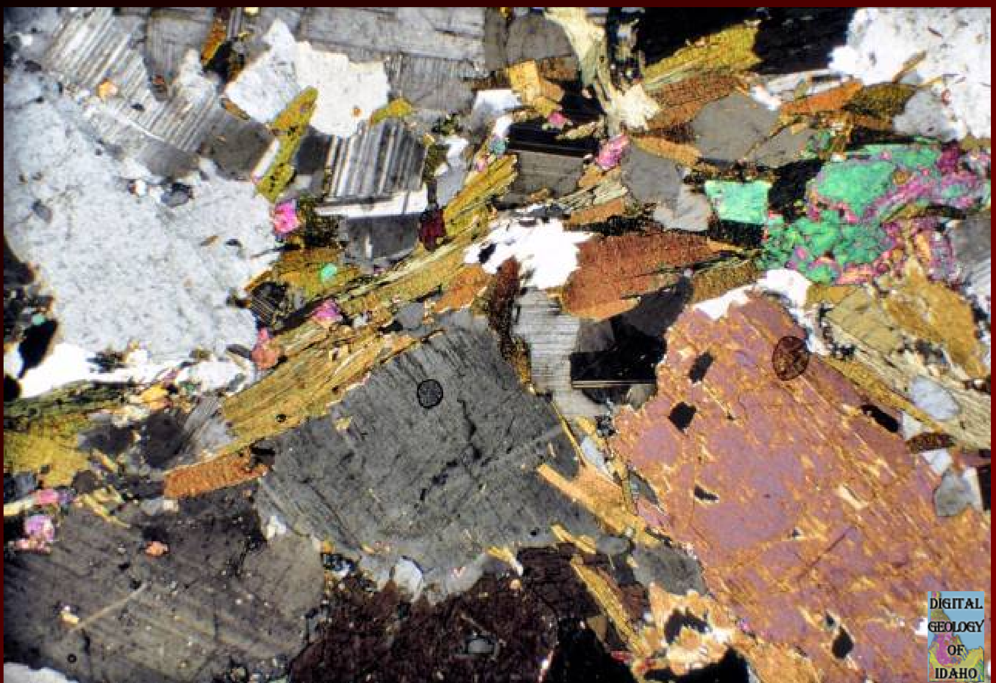
Thin section of Cretaceous-Jurassic hornblende-biotite quartz diorite. The twinned gray minerals are plagioclase feldspar. The biotite is the long green and brown mineral. Hornblende is the colorful mineral in the right side of the quadrangle.
