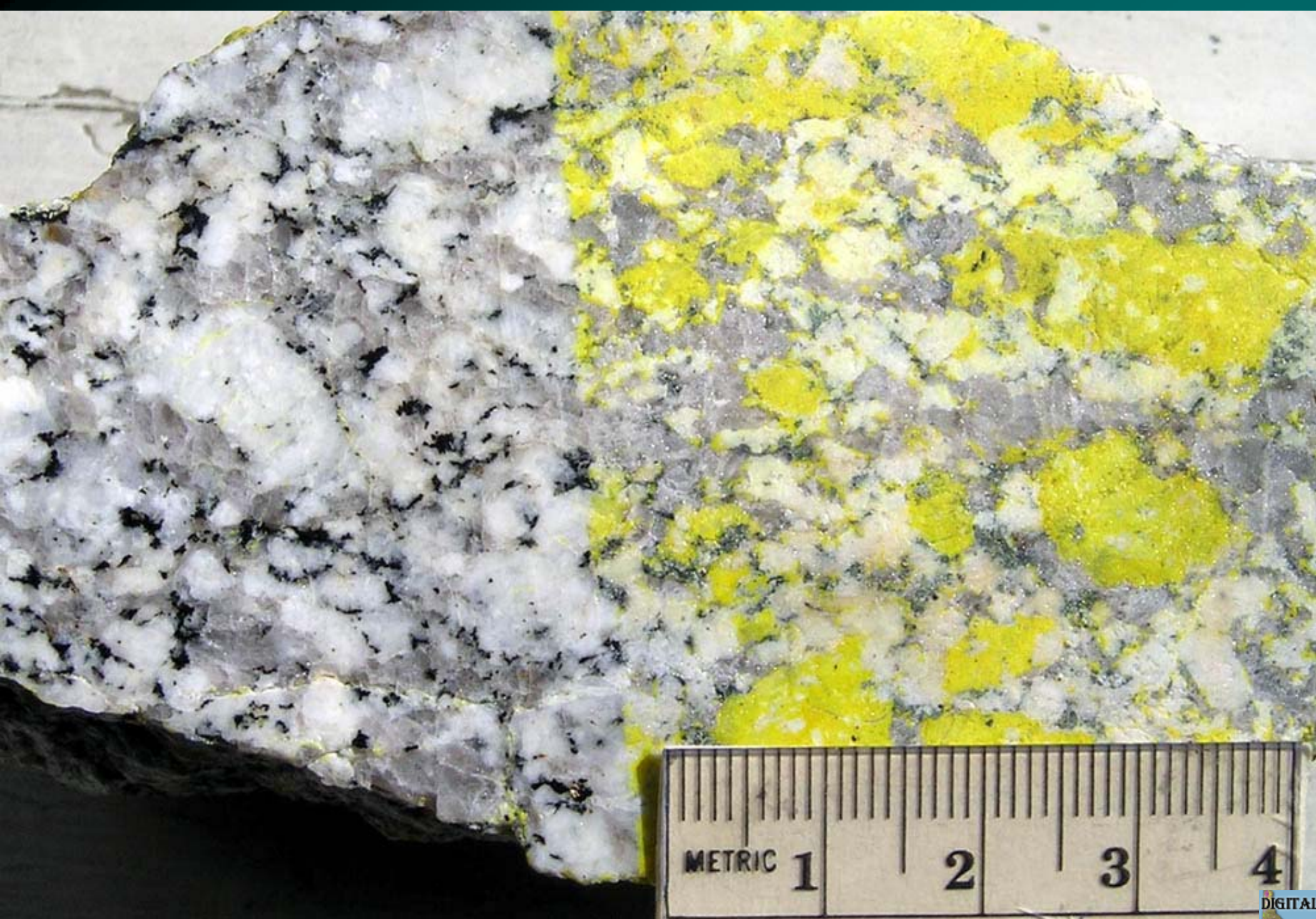
Stained slab of biotite granodiorite of the Bitterroot Lobe, Idaho batholith. Potassium feldspar is stained yellow. Plagioclase is white, quartz is gray.
