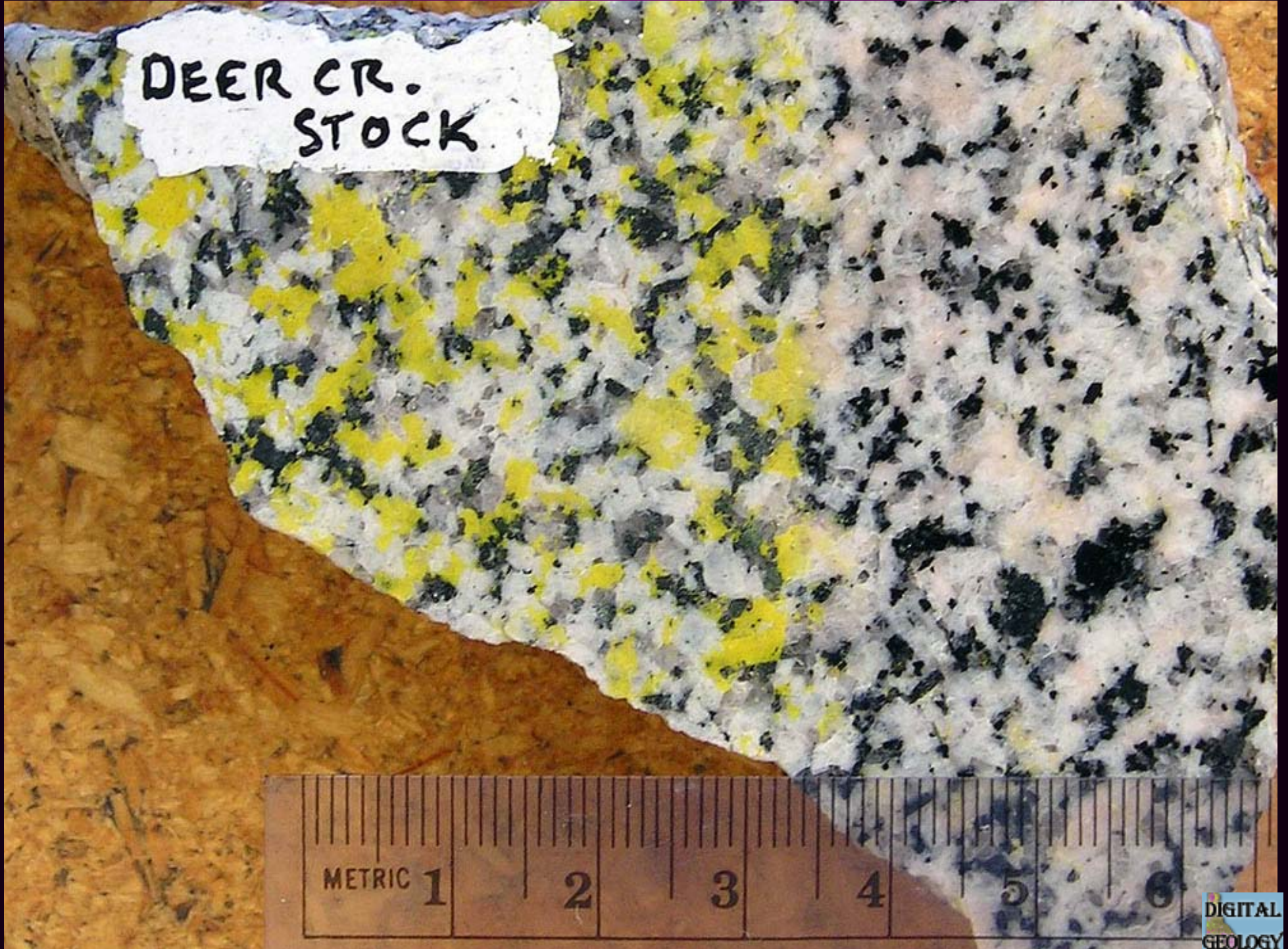
Granodiorite from the Deer Creek stock northwest of Hailey. Stained for potassium feldspar (yellow) on left side of slab.
