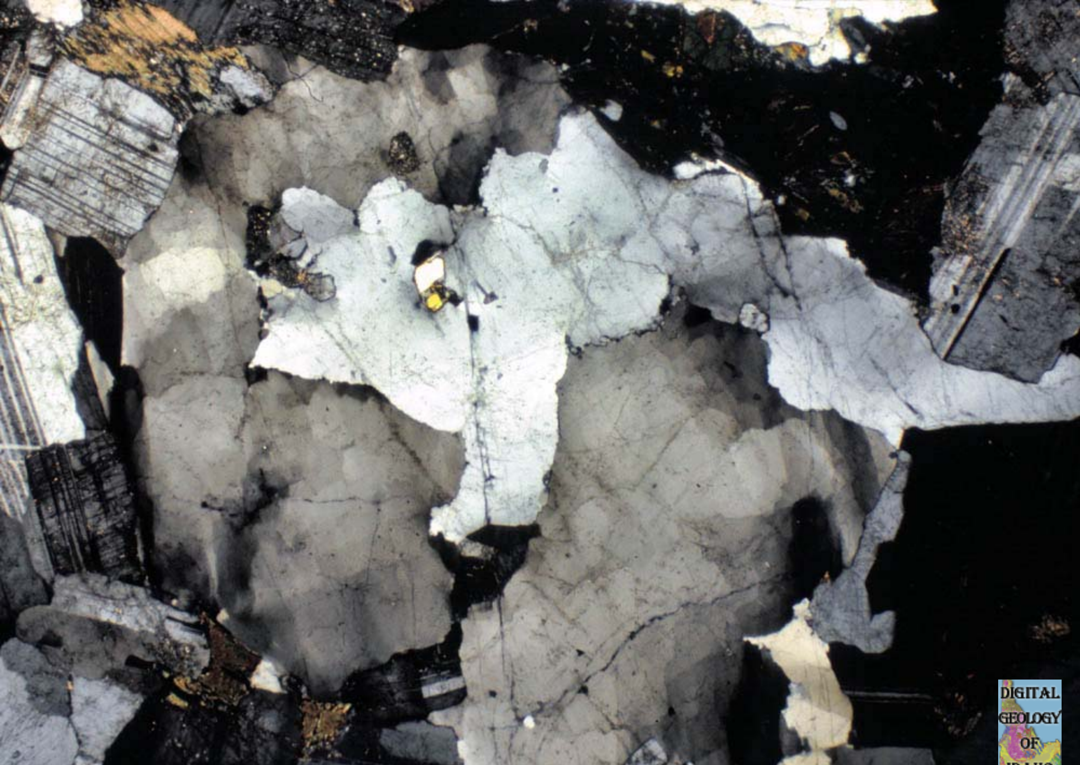
Thin section of typical biotite granodiorite showing strained quartz grains. Southeast of Big Smoky Creek. Plagioclase feldspar is twinned.
