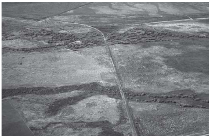
Figure 30. Wye in abandoned Gilmore and Pittsburgh railroad grade immediately southeast of Leadore. The view is to the west. The grade heads east at bottom of photograph toward view shown in Figure 31. The grade headed south on left side of view toward Gilmore (Fig. 29).
