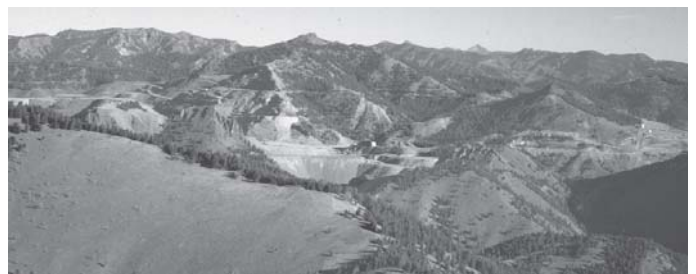
Figure 43. Aerial view looking northeast at the Thompson Creek open-pit molybdenum mine. The bare ridge in the foreground is underlain by Paleozoic Salmon River assemblage, which hosts the mineral deposit, near a Cretaceous intrusive body. The skyline behind mine is underlain by dacite lava flows of the Eocene Challis Volcanic Group.
