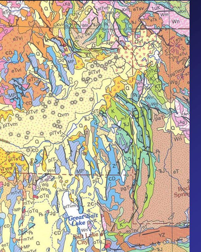
Geologic map of US from USGS. Shows thrust belt, basin and range, and SRP.
